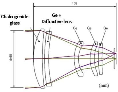
Fig. 3. Optical design of CIRC
