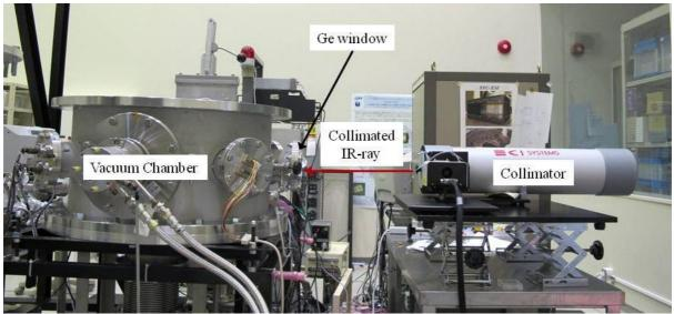
Fig.6. Configuration of the measurement setup
