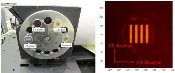
Fig.7. (left) 4-bar targets mounted on the collimator system. (right) Image of the 4-bar target taken with CIRC.
