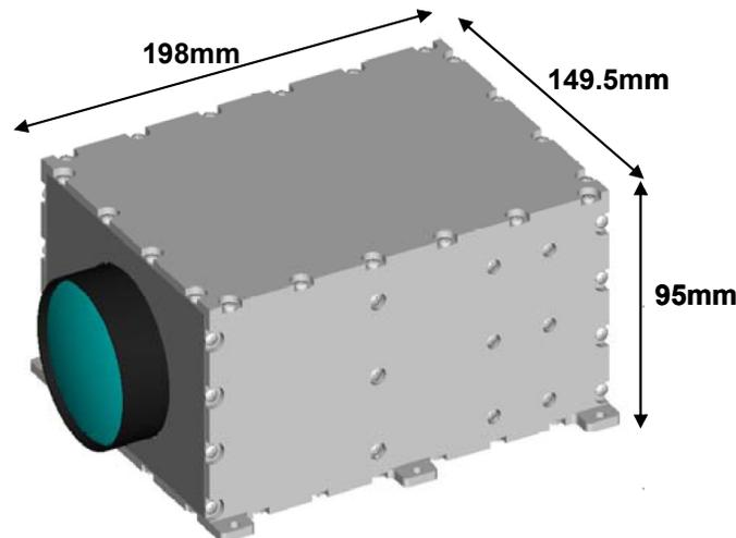
Fig. 3. Schematic view of the CIRC.
