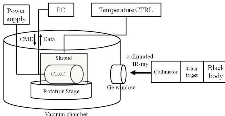
**Fig.5.** Schematic diagram of the experimental setup
