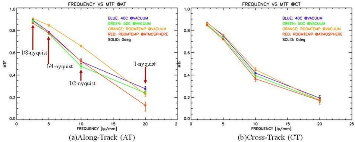
Fig.8. MTF of CIRC for the AT direction (a) and the CT direction (b).
