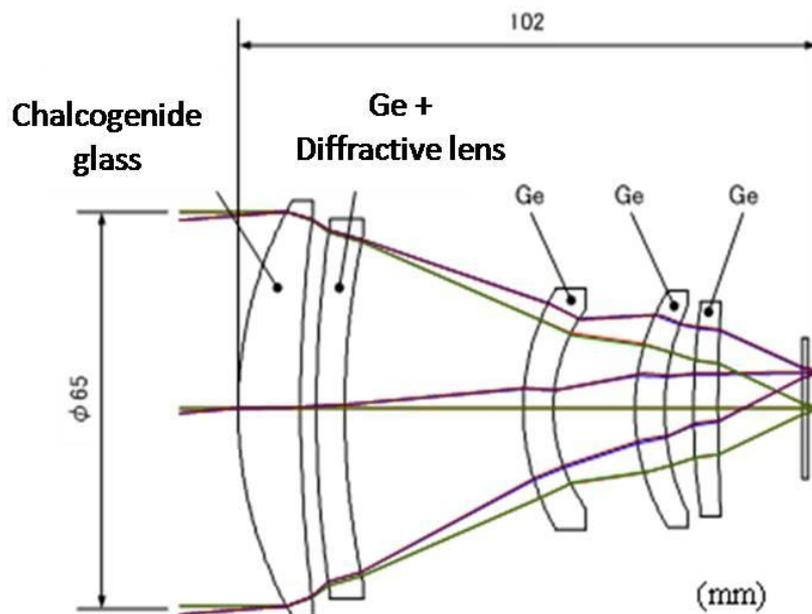
**Fig. 3.** Optical design of CIRC
