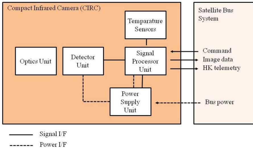
**Fig. 2.** System block diagram of the CIRC.
