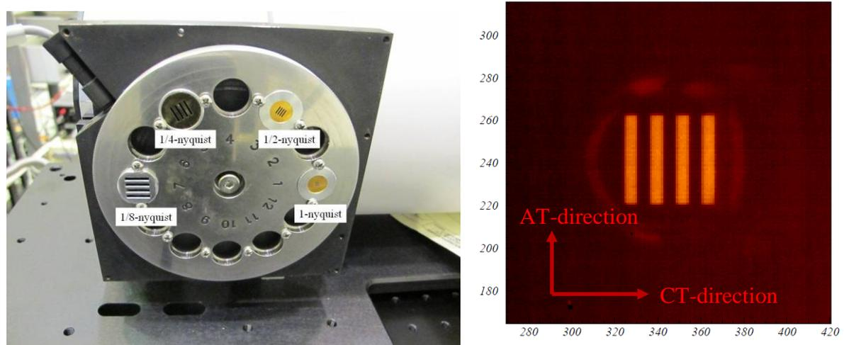
Fig.7. (left) 4-bar targets mounted on the collimator system. (right) Image of the 4-bar target taken with CIRC.
