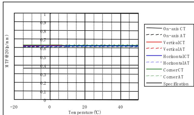
Fig. 5. Calculated MTF of the CIRC optics in the ambient temperature from -15 °C to 50 °C.
