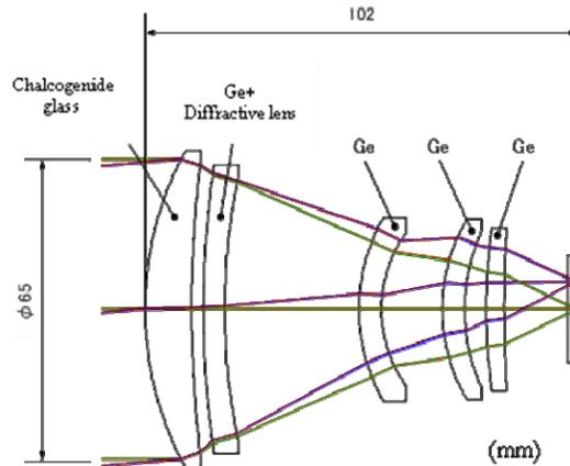
Fig. 4. Optical design of the CIRC.
