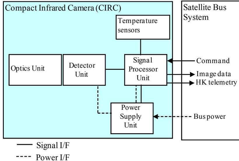
Fig. 1. System block diagram of the CIRC.
