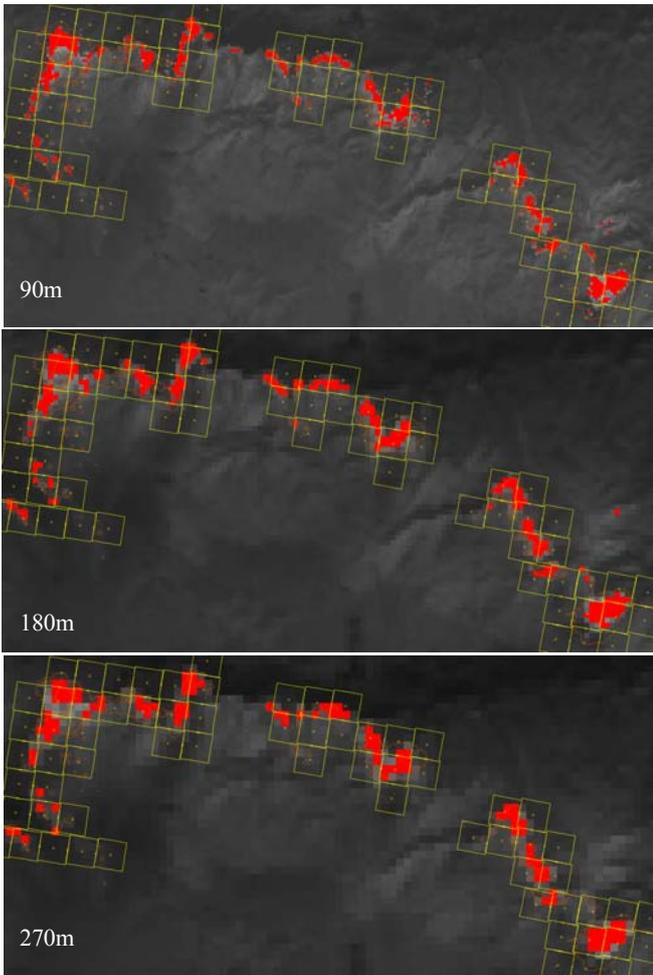
Fig 2. ASTER/TIR images of forest fire in California on October 26, 2003. The spatial resolutions are 90m (top), 180m (middle), and 270m (bottom). Red filled squares are the results of wildfire detection using thermal infrared data only. Yellow open squares are the results using MOD14.
