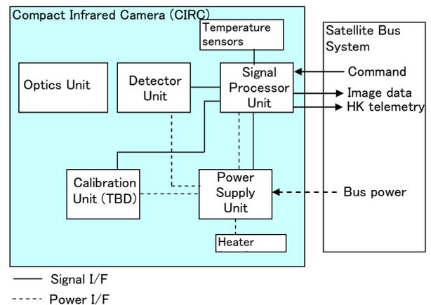
Fig 1. System block diagram of the CIRC.
